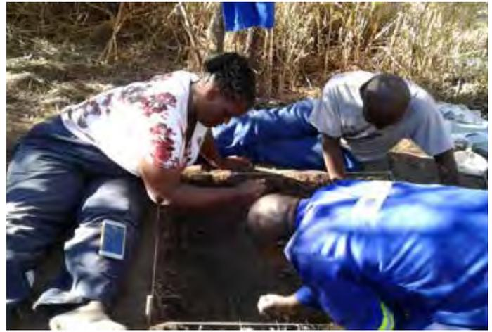
*Plate 2: Test pit excavation*
